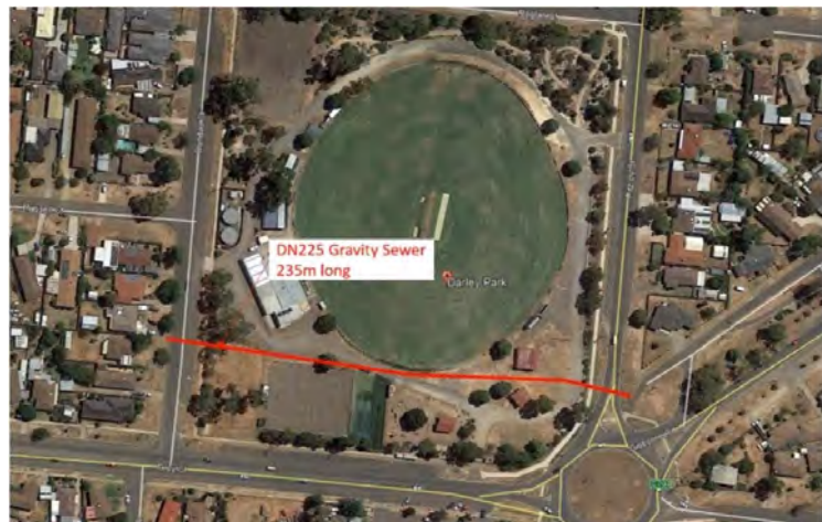
Map 4. The gravity sewer, see red line, runs east west across the south end of the Reserve
